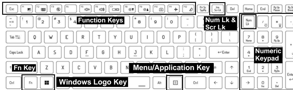
Figure 3 - (Factory Option) Full-size White-LED Keyboard
